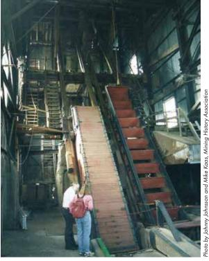
Michigan's Quincy Mine No. 2. The inclined shaft was 9,200 feet in length (6,400 feet vertical). A water bailing skip in the left shaft compartment was used to remove water from the mine.
