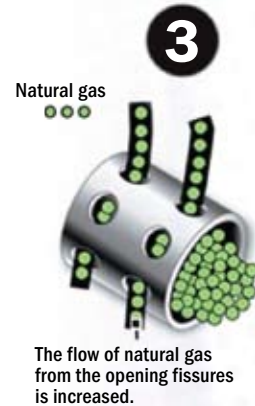
3. Increase Gas Flow The small fissures are widened by the pressure. The water mixture is pumped back out of the well and natural gas follows back up the pipeline to the wellhead.
